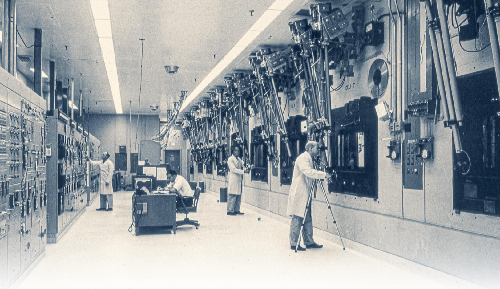
Scientists at Oak Ridge National Laboratory conduct research at a wall of Central Research-made telemanipulators. CRL became the international leader in the development of such instruments.
