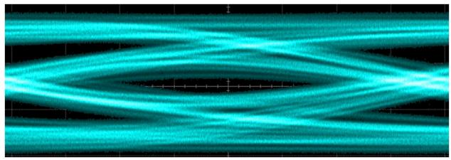
As can be seen in the second image, the clean "difference between high or low" has decreased dramatically, making the receiver introduce more errors in the data link. If the signal speed is increased too much, or the length is increased even more, the eye can completely close resulting in near 100% error rate. The figure below shows an example of this "closed eye" concept.
