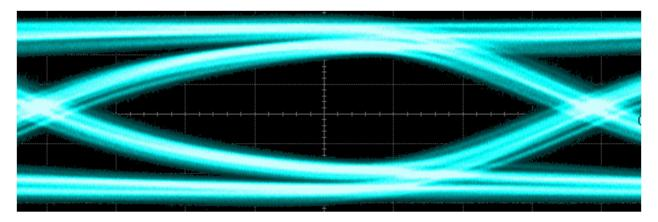
When a signal travels too far (or is increased in speed), the high frequency loses start to impact the edges of the signal and they take longer to reach the HIGH and LOW levels needed by the receiver.
