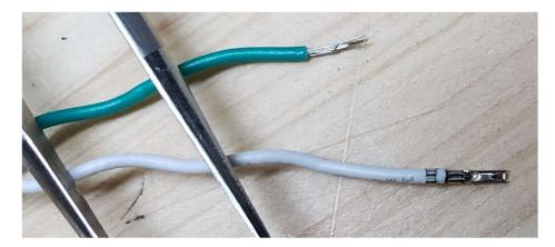
and now all you can hope for is to convert this cable into a USB2 only version as shown by removing cables 5, 6, 8, &9.
