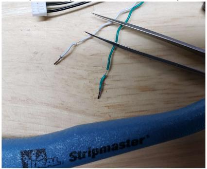
Be careful, and practice this first on some test sample wire. If you go too far with the stripmaster, you will strip off the crimp contact as shown:
