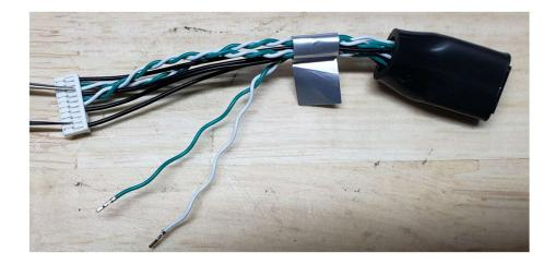
3) Use the stripmaster and very carefully open the insulation in each green and white wire about 15mm from the edge of the crimp contact. Only a 3-5mm section is needed to be exposed as shown:
