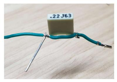
6) Repeat the soldering step, and again, once you are sure the joint is solid, trim back the rest of the radial lead, and then cut away the center cable "bridge" between the two radial leads as shown:
