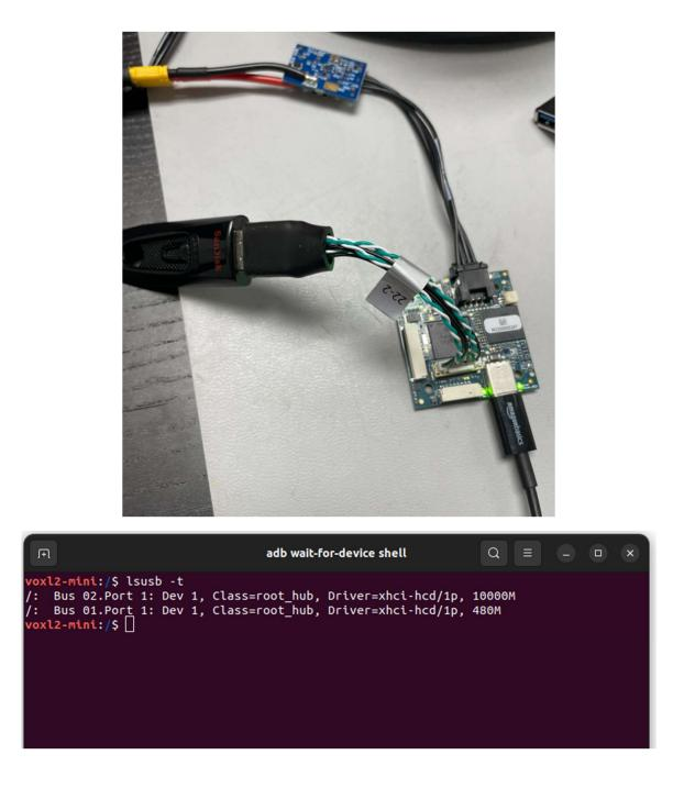
2) Then, we change out the MCBL-00022-2 for the MCBL-00022-AC and show the device does indeed now enumerate as USB3 as noted by the 5,000Mbps query:
