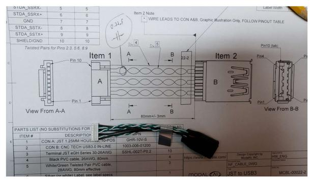
2) Remove the JST crimp contacts from the JST 10-pin shroud carefully, not damaging the plastic shroud since we need to re-use this. Normally, we recommend saving the pin at the expense of the shroud, but in this case, care must be taken to ensure neither are damaged. Use the tweezers to help gently remove the two cables, and then untwist the wires as shown:
