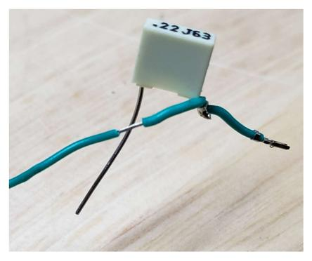
This method helps ensure the cap stays in place during soldering without the need for elaborate cable holders, but there are other ways to do this.
