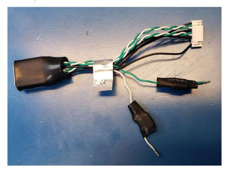
2) Then, using tweezers, insert the <u>white wire into the JST shroud at position 9</u> and the <u>green wire into the</u> <u>shroud at position 8</u> to recreate the original pinout from the drawing. An unmodified cable will help as a quick guide to make sure you have the wires back in their correct locations.
