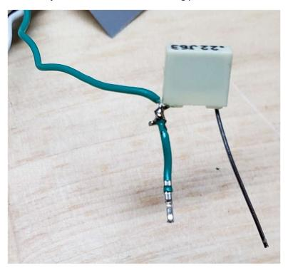
4) Now, the tricky part is to add a second insulation splice opening about 10-15mm away from the first lead further away from the crimp contact as shown:
