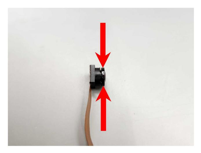
To focus the lens, it must be loose enough to be screwed/unscrewed into proper position. You should be able to do this with your fingers. Sometimes the glue residue will prevent adjustment. If that is the case, chip away the glue using a small flat head screw driver or something similar. Use caution to not damage the unit
