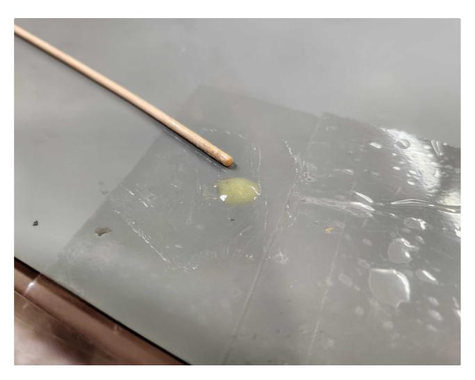
Cut your dowel so it has a sharp point as seen here. This will be used to apply the glue
