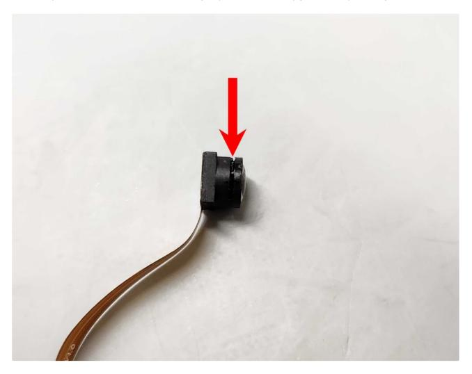
Glue is applied in between the sensor housing and the lens
