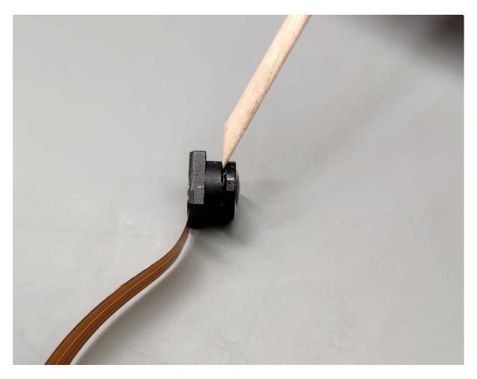
Put some glue on your applicator and dab it in between the lens and the sensor housing. Use extreme caution to not let any glue get on the lens
