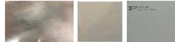
KITCHEN MATERIAL : COUNTER TOP : ARTIFICIAL STONE 12 mm. WHITE-GREY COLOR CABINET SURACE : LAMINATE HIGH-GLOSS WHITE COLOR & WOOD PATTERN
