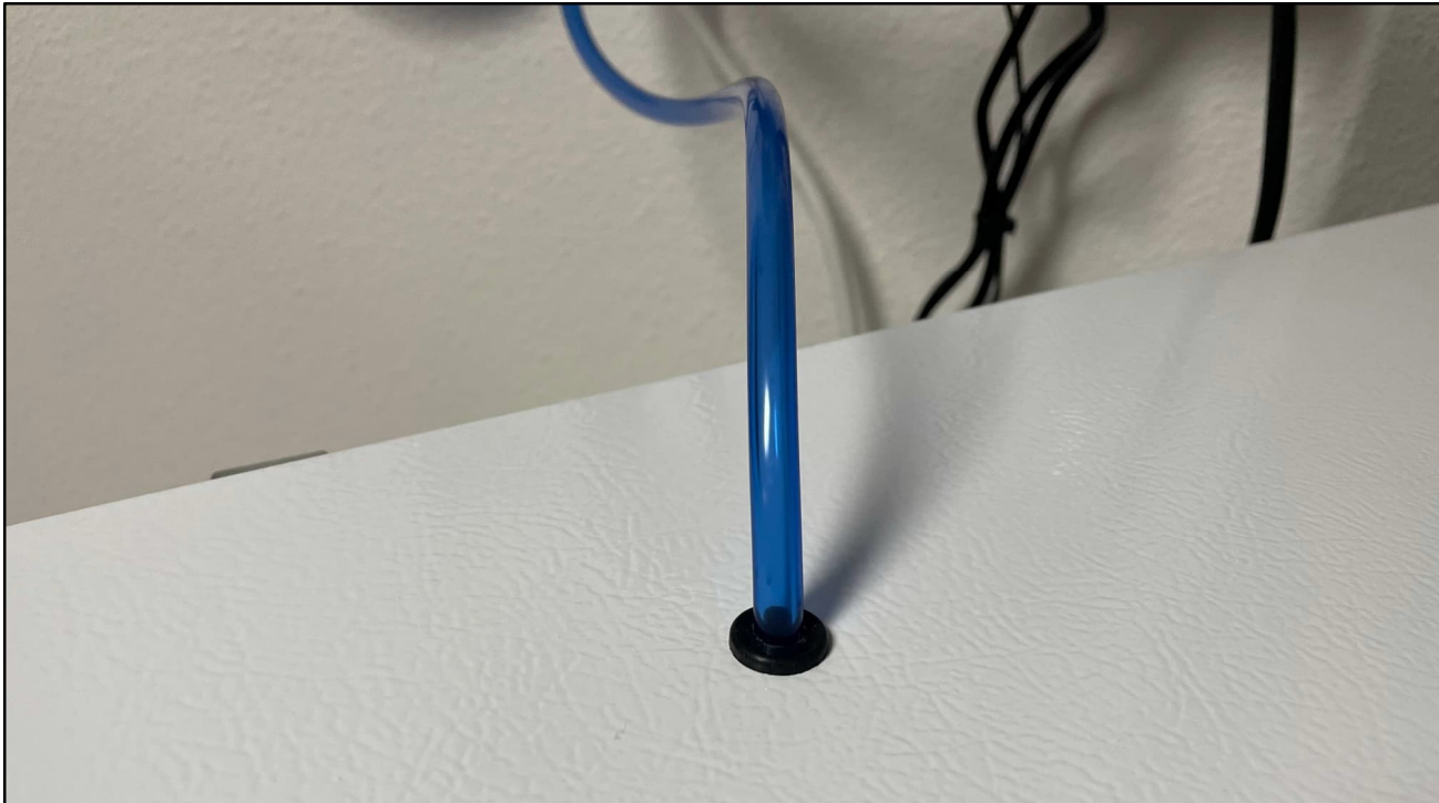
Top Hat grommet placed in a hole drilled through the lid.
