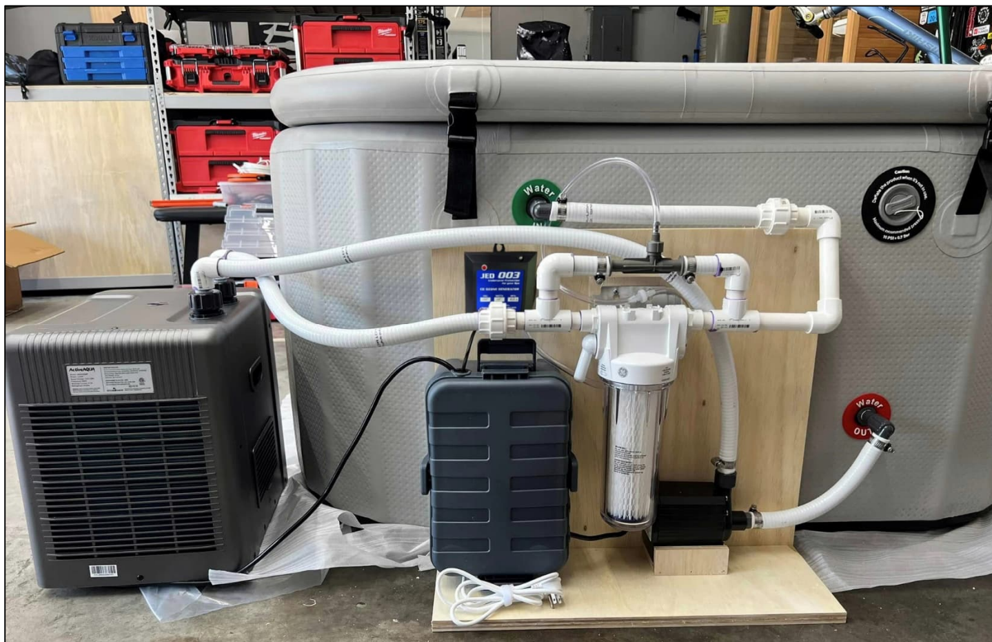
DIY cold plunge with chiller, inflatable tub, pump, filter, and JED 003
