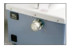
Unscrew the clear plastic filter cover counterclockwise. Remove the white filter and any micro crystals by wiping and/or tapping the filter element on a counter to loosen them. If the filter is grey in color instead of white, it should be replaced. Replace filter and tighten the filter cover snug, making sure the O-ring is evenly seated in the rim of the clear filter cover.
