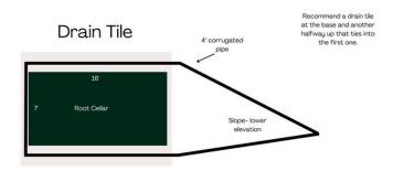
Step 5: Fill in the hole with 2"-3" stone close to the cellar and pea gravel outside of that closer to the edge of the hole. (See image below) \* An experienced dirt worker will be able to manage layering the stone so the larger stone is close to the cellar and the pea gravel is closer to the outside. If you are not using a dirt contractor and are doing it yourself, you could use just the larger stone to fill the hole.
