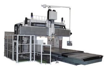
The MCR-BIII Double Column boasts an unmatched table size of 79" x 149" with a max load of 48,500 lbs. Its ability to travel X 157.48", Y 100", Z 31.496", W 39.37" combined with the 50 magazine automatic tool changer will make quick work of large, intricate parts while maintaining the tightest tolerances.
