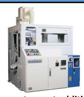
Our most recent addition is the Nishijimax NHC-110 NC CNC Cutting Machine which can cut material flat within an industry leading .002" and overall length tolerance ±.005".
