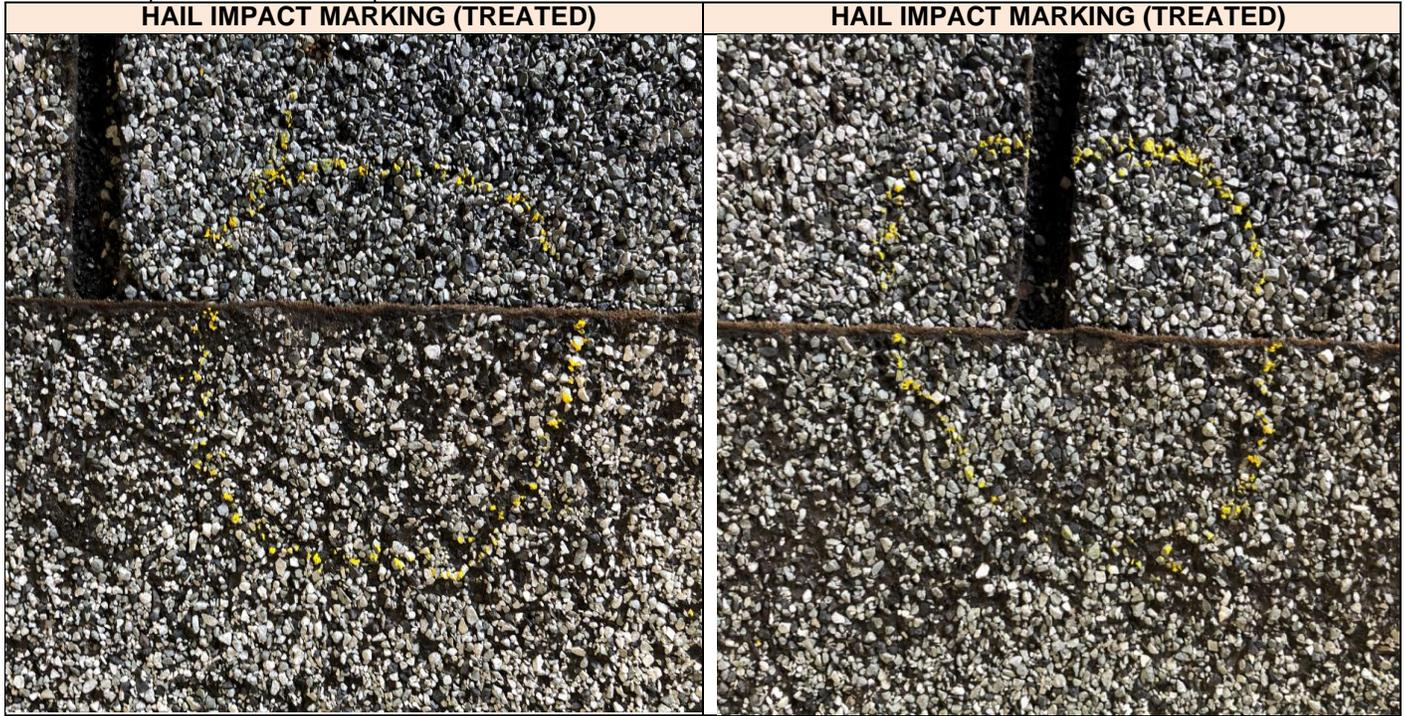
**A6 Hail Impact Steel Ball Test per UL 2218 on Treated Material**
