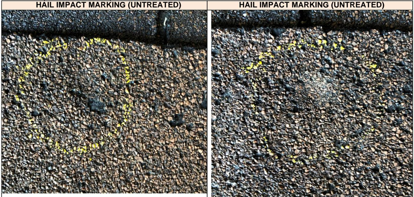
**A10 Hail Impact Steel Ball Test per UL 2218 on Untreated Material**
