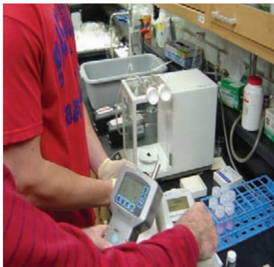
Figure 7–3. Combined use of the OPC, CPC, and two filter samples to determine the presence of nanomaterials
