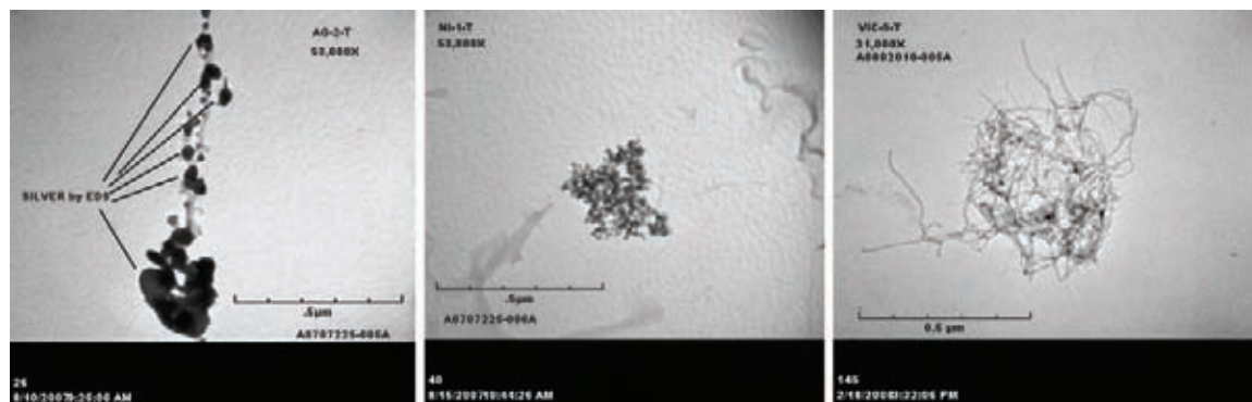
Figure 7–2. Photomicrographs of airborne engineered nanomaterials (airborne samples of engineered nanoparticles of silver, nickel, and MWCNT analyzed by TEM and EDS)
