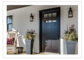
Remove existing 3-0/6-8 entry door and jambs and replace with new 20-gaugesteel unit, including clear, dualpane half-glass panel, jambs, and aluminum threshold with composite stop. Door is factory finished with same color both sides. Exterior brick-mold and 2.5-inch interior colonial or ranch casings in poplar or equal prefinished to match door color. Replace existing lockset with new bored lock.
