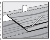
Fill any expansion spaces around potentially wet areas (such as refrigerators, tubs, etc.) with premium, waterproof 100% silicone sealant.
