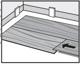
Product Description: Rigid Core Plank and Tile Flooring **Grade Levels:** Above Grade / On Grade / Below Grade Installation Method: Floating - Drop and Lock
