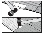
After installing the last piece of the second row, slide the entire assembly against the spacers on the starting wall, maintaining the required 1/4" (6mm) expansion
