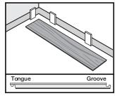
Interlock the next plank at the end joint of the first plank by inserting the tongue into the groove of the adjoining planks.
