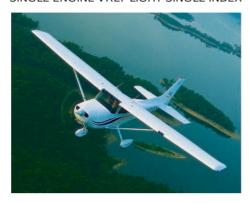
The Cessna 172 Skyhawk is an American four-seat, single-engine, high wing, fixed-wing aircraft made by the Cessna Aircraft Company. First flown in 1955, more 172s have been built than any other aircraft. It was developed from the 1948 Cessna 170, using tricycle undercarriage, rather than a tail-dragger configuration.
