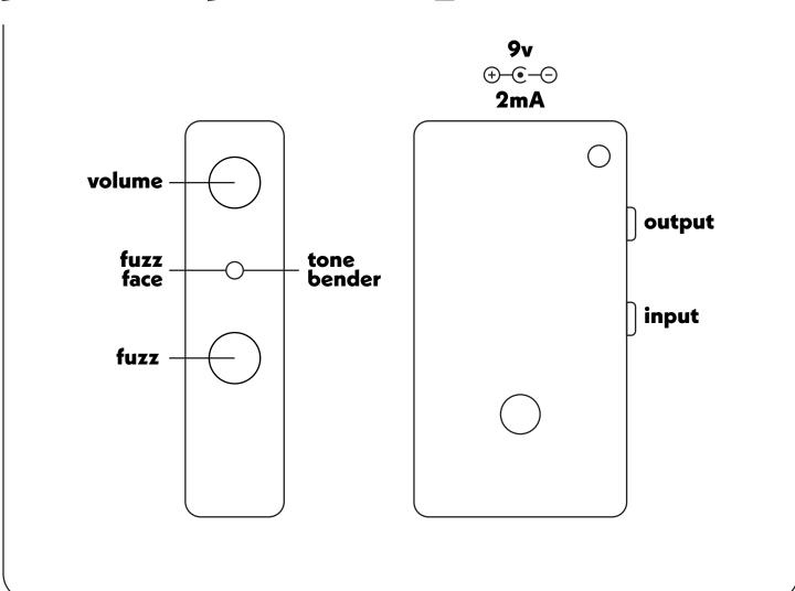
it is recommended that this pedal should be situated before any buffered effects in your signal chain. the closer this pedal can sit to your instrument the better. however, your ear is the ultimate authority on whether or not this placement sounds best. run this pedal only at 9v using a standard center negative power supply.
