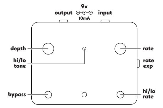
depth: this blends the effected signal in with the bypass signal.
