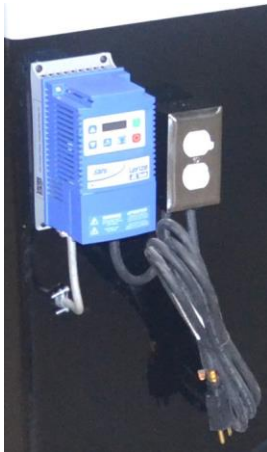
Variable Speed, Timer Switch , Receptacle for solution pump and corded plug included
