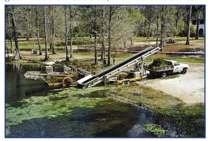
removal harvesters are powered by side-mounted paddle wheels which operate independently in forward or reverse. As a result, these harvesters are highly maneuverable around docks and boat houses. Also, the machines can operate in as little as 12 to 18 inches of water. These harvesters cut plants off at depths of 5 feet and in swaths 8 feet wide with a hydraulically operated cutter head and convey the cut plants into a storage bay on the harvester. When
