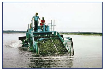
mechanical control in the US. The first machines were developed in the 1950s by a Wisconsin company to harvest Eurasian watermilfoil and curlyleaf pondweed from the edges of the hundreds of lakes in the Upper Midwest. These lakes are generally deep in the middle and aquatic weeds naturally grow in the shallow littoral areas, which receive intensive use for swimming and docking. Harvest and
