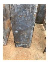
Class 3 – Pans have been oiled and maintained with multiple uses. Concrete is building up but not excessive.
