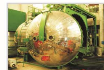
德国技术全自动真空浇注罐 Full automatic numerical steam vacuum gating systems from German
