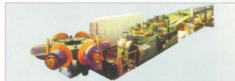
德国GEORG公司全自动铁芯生产线 Full automatic production line of iron core imported from GEORG of German
