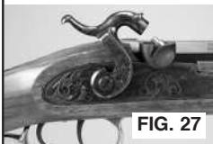
CAP LOCK HAMMER IN "COCKED" POSITION
