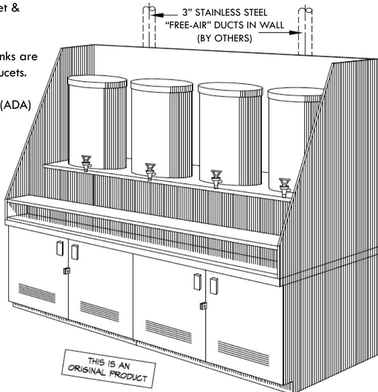
SEE CATALOG PAGE #2-28A FOR THE EXACT LOCATION FOR THE "FREE-AIR" DUCTS ENTERING THE BASE CABINETS
