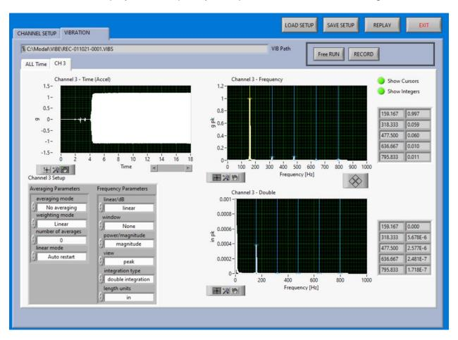
In the display above, CH 3 shows the time signature response along with the frequency content and the double integration of the response to displacement. These calculations are performed in real-time during collection. When cursors are enabled, they will display frequency and magnitudes. The integer cursors are useful to monitor harmonics.
