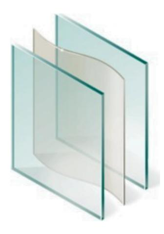
**Laminated Glass**: This glass type is not only more robust than standard glass but also classified as Safety Glass. It features an interlayer positioned between two glass layers, often composed of a clear plastic called polyvinyl butyral (PVB). This PVB interlayer serves multiple purposes, such as preventing the glass from shattering when broken and providing excellent vibrationdampening qualities, making it excellent choice for an soundproofing.
