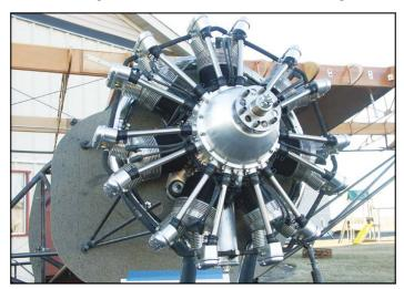
The Rotec Engineering R2800 radial engine now adorns the front of the Ace. A wooden propeller is on order from Culver Props. I am now working on the various complexities of engine installation. She is about 90% done and 90% to go.
