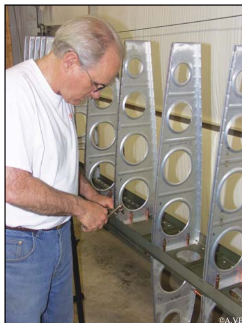
Steve "Clecoing" ribs in place before riveting.
