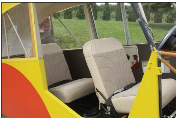
The seats, refurbished by Lorraine Morris, are installed.
