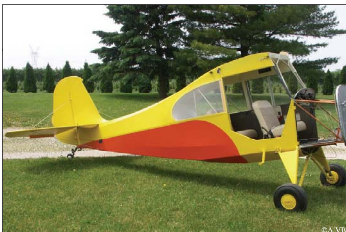
The empennage and landing gear are installed.
