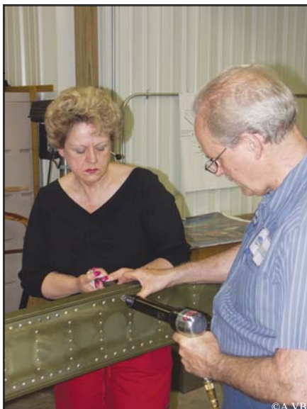
Steve and his wife Jan (a.k.a. Rosie the Riveter) installing rivets in the spar.
