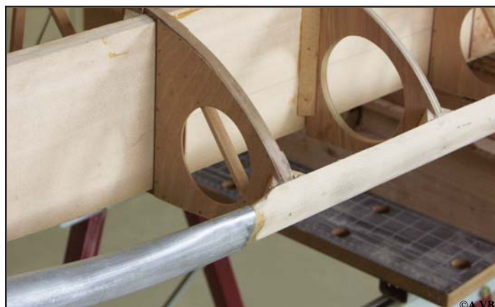
Wing tip tubing to leading edge junction
