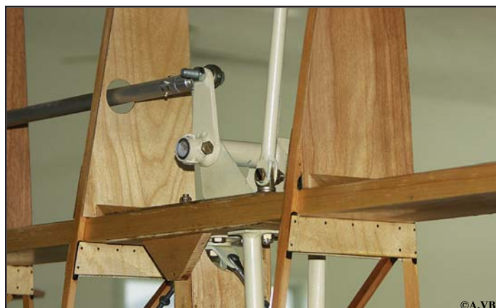
Aileron linkage detail
