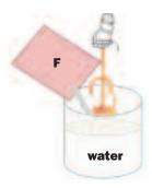
The product should be mixed in a forced action mixer or in an appropriate sized metal or plastic drum using a slow speed drill and a spiral paddle. The water should always be placed into the mixing vessel
