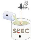
Both of the components should be briefly stirred to ensure that any settlement products are fully suspended. Empty the entire contents of the curing agent into the base component. To ensure that
