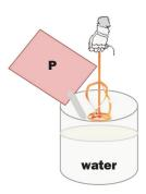
Place 2.3 litres of water into the mixing vessel and with machine mixing, slowly add the bag of **SpECtop CRM** and mix for 3 minutes until fully homogeneous. Do not mix for longer than this period
