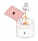
In a clean mixing vessel pour the total contents of the liquid component and slowly add the powder component whilst mixing using a slow speed drill (300 rpm) and paddle. Mix until smooth consistency is obtained (2-3 minutes). Leave to stand for 10 minutes and remix.
