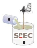
The entire contents of the curing agent should be emptied into the base component, ensuring that the sides of the curing agent tin are carefully scraped to remove all the material.
