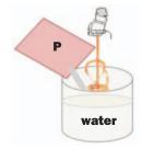
Pour the measured volume of water into an appropriately sized plastic or metal drum. The powder should be added to the water slowly whilst
