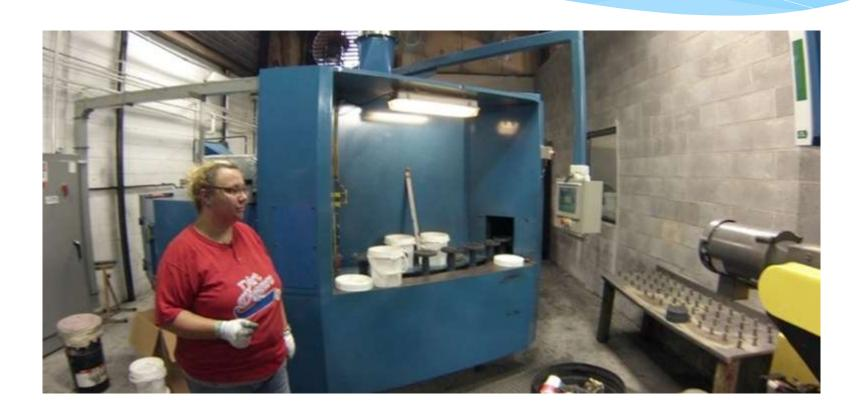
Dainichi Techno Turn – DL65 x 3000, 17-3/4" chuck, 25-1/2" swing over bed, 118" between centers w/ 3-1/4" spindle throughput. Fanuc 21T.
