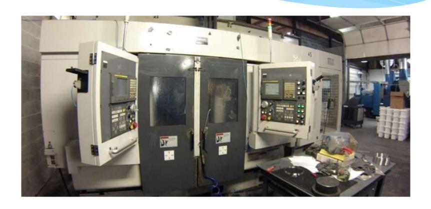
FUJI ANW-4100 – Twin Spindle Lathe – Robotic Loader and Q.C. separator. Capable of running as two programmable independent lathes.
