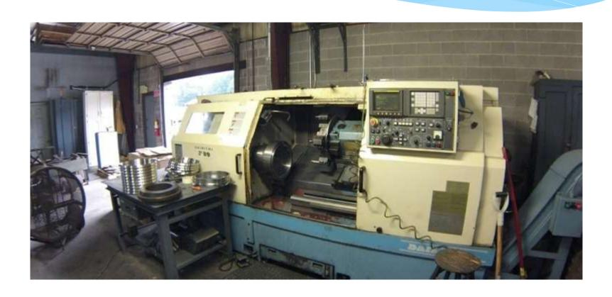
Dainichi F35 x 1250, 15.75" Hydraulic power chuck, 16.5" max turn, 21.7 swing over bed, 50" between centers, Fanuc 21T.
