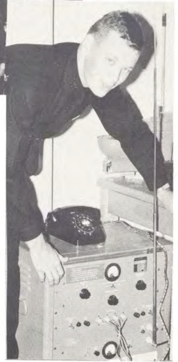
Mid'n Langley prepares to operate radio controlled ship steering and navigation trainer.
