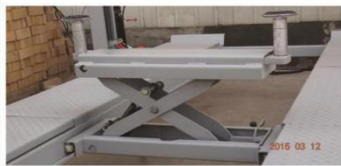
二次举升 Secondary lifting
