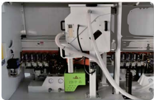
Upper Gluing Pot Gluing System +Fast Melter Glue
