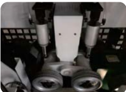
Pneumatic hold-down feeding wheel can adjust the pressure in sections, which is beneficial to the smooth feeding of wood with different thickness.
