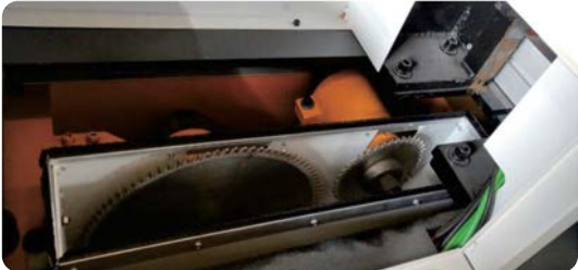
Taiwan brand guide rail, durable, high precision, and the error within 0.01mm per meter, Taiwan DELTA Brand servo motor, higher precision, more sensitive, Main saw blade and scoring saw blade are controlled by independently,
