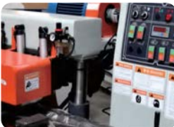
The unique powerful feeding system is more conducive to the synchronous feeding of the upper and lower feeding wheel group so as to maintain the smooth feeding of the processing process.
