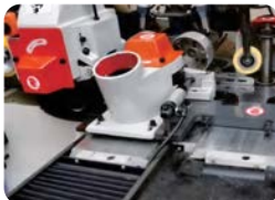
#Equipped with shaft cooling function , it can increasing the life of saw blades and ensure the precision of cutting. #Suction inlet: Lateral protection safety device, equipped with central vacuuming, effective discharge of sawdust keep working environment clean.
