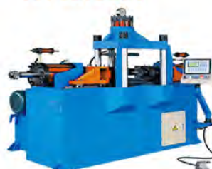
Pipe end forming machine TM-50T2S90°
