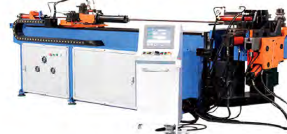
Three-dimensional CNC bending machine (Left bending machine)
