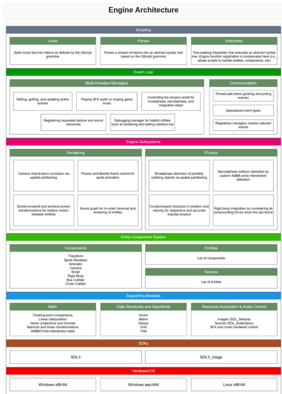
Figure 2: Provided is an example game engine architecture. Students document every component to reinforce how the components fit together, and iterate on their game engines.
