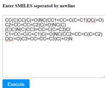
Figure 66. Inserting structures in SMILES identification format. Each SMILE must be separated by newline.
