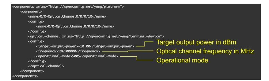
Full configuration example using NETCONF: https://xrdocs.io/design/blogs//zr-openconfig-mgmt
