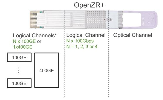
Note: OpenZR+ MSA specification also supports 200G mapping over 200G-400G logical channels
