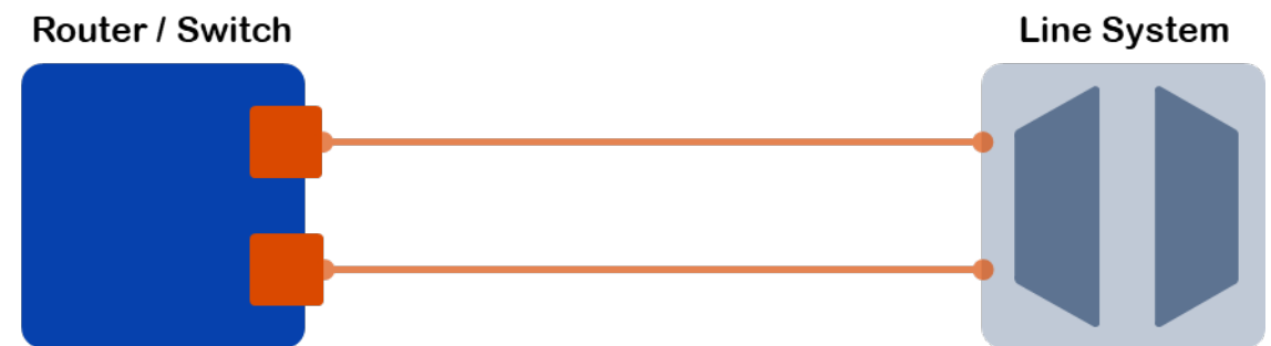
Router-based DCO (IP-over-DWDM)
