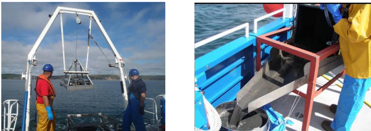
Figure 31. Mini-Hamon grab (left), and equipment for sieving benthic fauna samples (right). Images taken from Godsell (2019).
