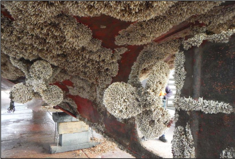
Figure 18: Ficopomatus enigmaticus on hull of workboat in Southampton Water, berthed adjacent to Marina 3 (SMQ). Image: © Rob Holland.
