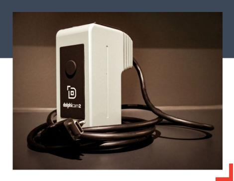
The transducer connects to the dolphicam2 Black Box through a standard USB C cable which handles power, control signals and data. The unique 128x128 "crossed electrodes" transducer creates a grid of 16,384 individual ultrasonic echoes ("A-scans") over the 32x32mm transducer area, which makes it capable of detecting very small defects.
