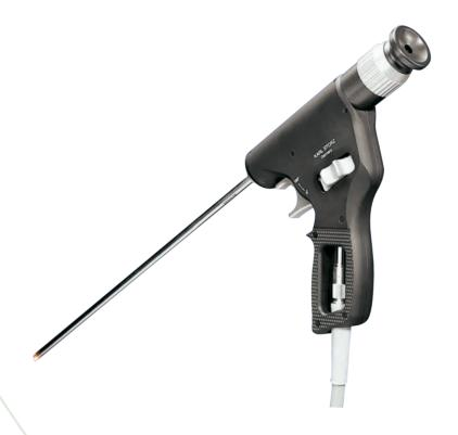
The so-called swing-prism borescope features a swing prism at its tip. Using a control handle, the direction of view can be infinitely adjusted between 0° and 140°. In addition, the sheath can be rotated by 400°. This provides you with the best possible field of view.
