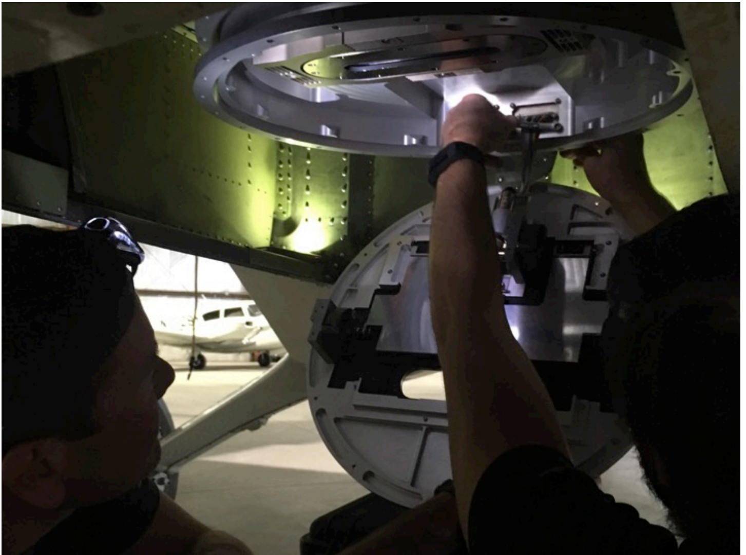
Abe and Mitch repair NIS Shutter failure in D05
