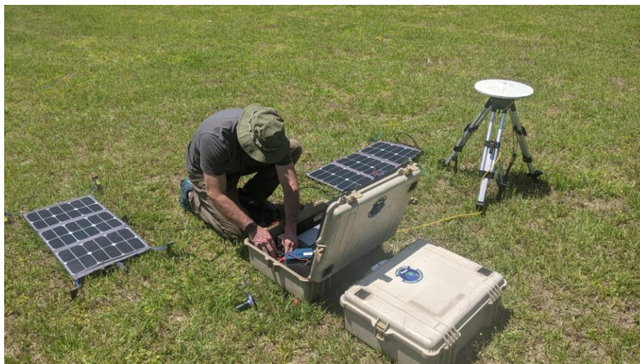
ASO Abe Morrison repairing LENO GPS station. Pic by Cam C.
