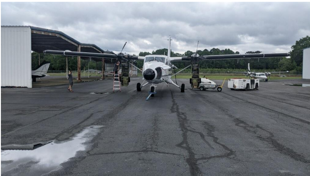
Engine run ups being conducted at the conclusion of corrective maintenance. Pic by Cameron C.
