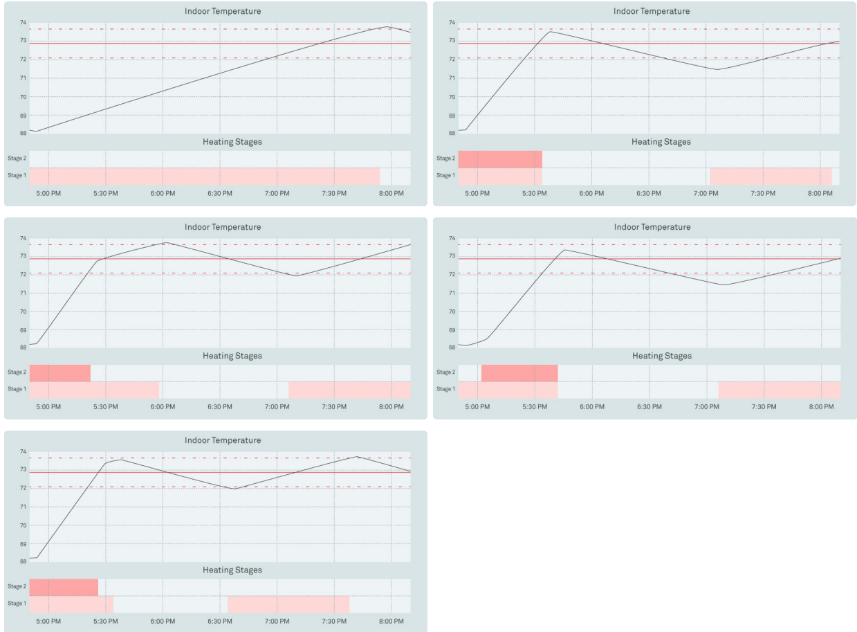
Figure VI: Example control approaches that HVAC Control 2.0 evaluates in its search for the optimal control for a scenario where the setpoint has just been increased by over 4 °F. It tries out (a) only stage 1 heat, (b) only stage 2 heat, (c) running stage 2 heat and then stage 1 heat, (d) running stage 1 heat and then stage 2 heat, and (e) running stage 2 heat, then stage 1 heat, and stopping early to avoid overshooting.
